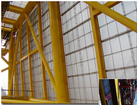
Ladder Heatshields protecting SALTIRE drilling derrick
