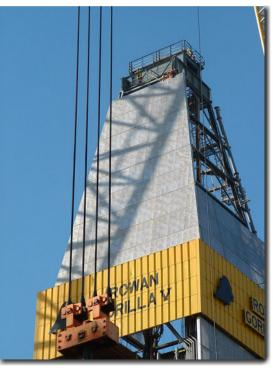
Locker Radiant Heat Shield cladding panels were specifically developed for the safety and protection of personnel and equipment against radiant heat from flares on Oil Rigs and FPSO's.
